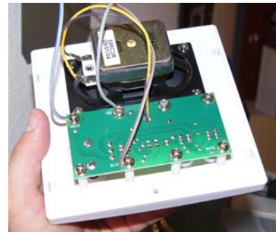
Figure 7 - Room Station Wiring - 3-Wire
